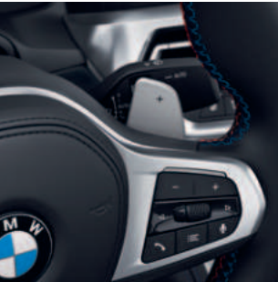
■ The 8-speed Steptronic Sport transmission offers incredibly sporty gear changes. Whether automatic or manual using gearshift paddles or selector lever.
