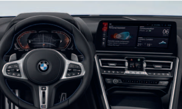
□ BMW Live Cockpit Professional includes two high-quality displays consisting of a 12.3" Control Display and a fully digital 12.3" instrument display.
