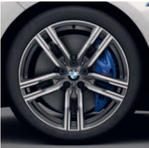
■ 19" M light alloy wheels Double-spoke style 727 M Bicolour Orbit Grey with mixed tyres and run-flat tyres, gloss-lathed, wheel size front 8J x 19 with 245/40 R19 tyres, wheel size rear 9J x 19 with 275/35 R19 tyres.
