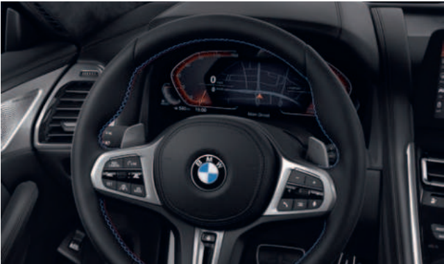
□ BMW Live Cockpit Professional includes two high-quality displays consisting of a 12.3" Control Display and a fully digital 12.3" instrument display.
